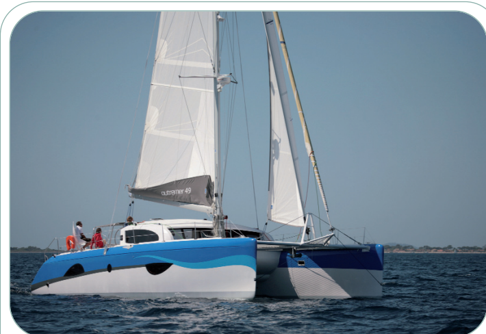
Powerful bows, barely immersed forefoot, well proportioned coachroof: the 49' is intended for the open sea.
